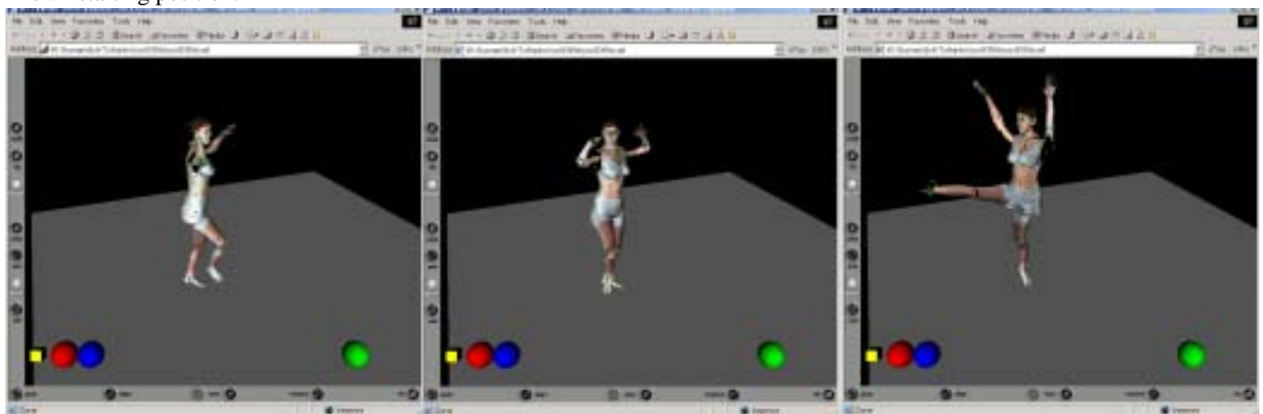
Figure 4 Three frames of a motion capture sequence from BVH file controlling a CAESAR body in VRML browser.
